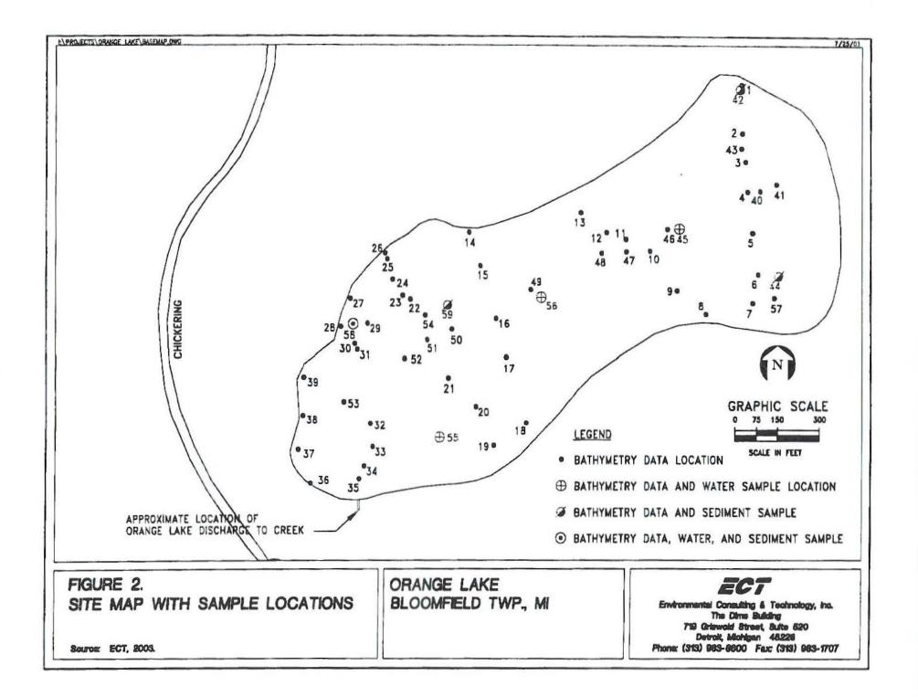
The sediment samples collected were focused on the unconsolidated muck that exists above the native lake bottom. Sampling methodology was designed to screen the overall sediment layer. Sample locations were located using GPS and are shown on Figure 2.
