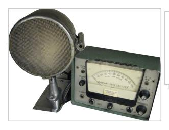
**Left,** There was a time when this radar unit was state of the art speed measurement equipment! The large antenna to the left was hooked to a patrol car's passenger window. Everyday, the unit had to be calibrated before patrol using the tuning forks (below).
