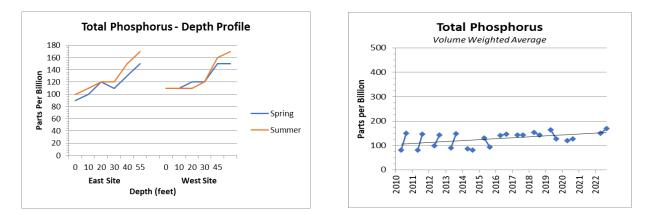
Additionally, we used the concentration of phosphorus and the lake volume to calculate the total phosphorus load. This quantified the amount of phosphorus in the lake. The following graph shows the results of this calculation over the years of our testing. The old adage states 1 pound of phosphorus can support 500 pounds of plant growth, so the spring average load of 547 pounds of phosphorus could support almost 136.75 tons of plants!
