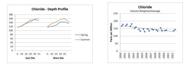
Finally, we used the concentration of chloride and the water volume of the lake to calculate the lake's chloride load. The following graph shows the results of this calculation over the years of our testing. This quantified the amount of chloride in the lake.
